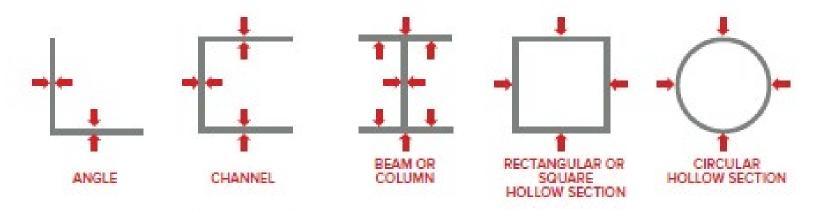
Figure 6: Pictorial guide for locations of DFT readings
