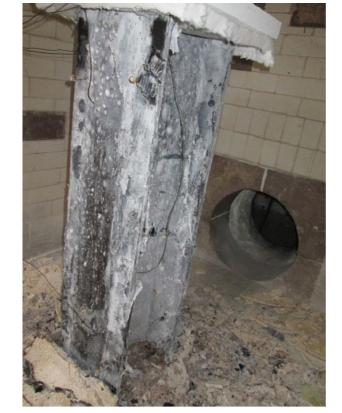
BASIC 250UC73 COLUMN (90 X 45 TIMBER FRAMING)
